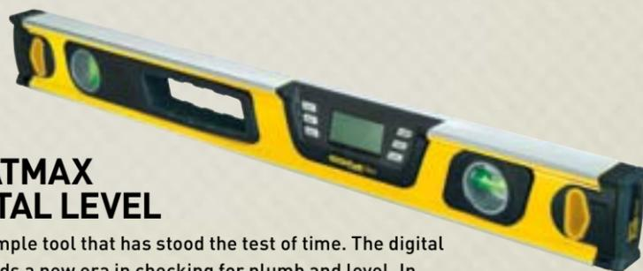
The spirit level is a simple tool that has stood the test of time. The digital level, from \$80, heralds a new era in checking for plumb and level. In addition to bubble vials, the tool beeps when it's horizontal, vertical, or at 45°. It also features a backlit LCD screen, and shows the exact tilt with a precision of 0.1°. It can be switched to show percentage gradient and rise over run, and has magnetised edges. [stanleytools.com.au](http://stanleytools.com.au)
